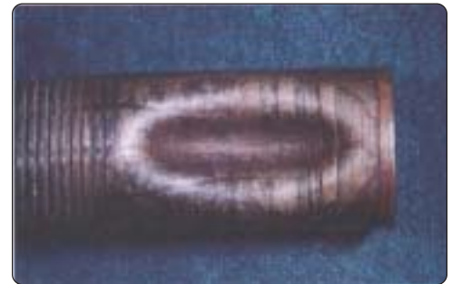
Fig. 6. Collapse of evaporator tube because of freeze-up.
