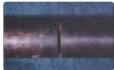
Fig. 3. Velocity-induced vibration of tube.
